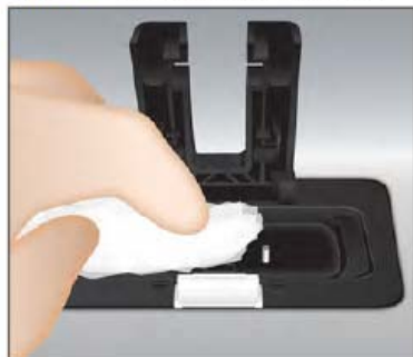
Figure 14 Dry the Wash Reservoir
