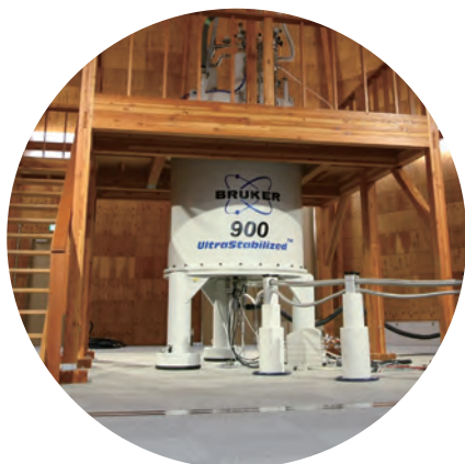
900 MHz NMR spectrometer
